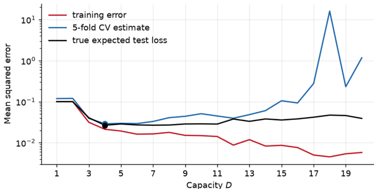
Figure 17: Five-fold cross-validation choosing the capacity of the simplified model from one training set of I = 30 points. The training error (red) falls, not quite steadily, as capacity grows and would always choose a big model. The cross-validation estimate (blue) is computed from the training data alone, yet its minimum (marked) lands at the same capacity as the minimum of the true expected test loss (black), which we can compute only because we know the generating process. The cross-validation curve sits above the truth because each fold trains on just 24 points. For the same reason it explodes from about D = 15 onward: each fold’s fit is approaching its own interpolation threshold, D + 1 = 24 , and is climbing the double descent peak of fig. 16.
